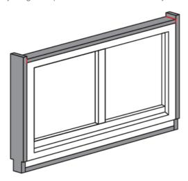
**Step 5:** Use OTTOTAPE Trio-FBA for the window connection joint and stick it on.
