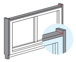
**Step 4:** Stick OTTOTAPE Trio-BKA MF1 onto the lintel and the balustrade, leaving a small lateral overhang (adhesive joint). Cutting out/adjusting the tape at the window connection joint or other substructure profiles.
