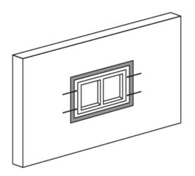
Step 6: Place the window frame into the opening, adjust and fasten.
