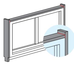
**Step 4:** Stick OTTOTAPE Trio-BKA MF1 onto the lintel and the balustrade, leaving a small lateral overhang (adhesive joint). Cutting out/adjusting the tape at the window connection joint or other substructure profiles.
