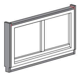
Step 5: Use OTTOTAPE Trio-FBA for the window connection joint and stick it on.
