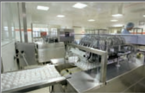
Production of influenza vaccines: The hatching eggs are inoculated with a solution containing the virus.
