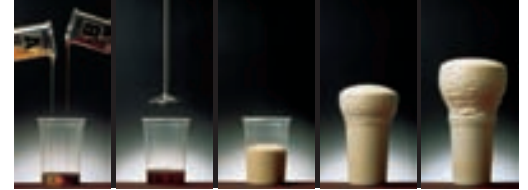
The reaction phases of hard polyurethane foam: When the two-component mixture is foamed up the volume increases around 25-fold.
