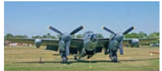
Lightweight sandwich components for the military aviation industry in the 2nd World War like those made from wood materials for the Mosquito fighter planes.
