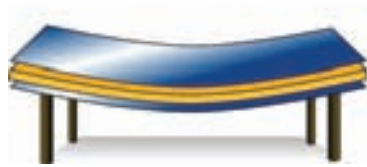
Loose layers bend under their own weight alone.
