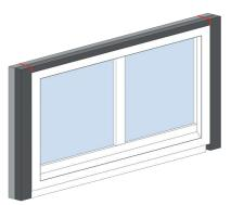
Step 4: Stick OTTOTAPE Trio-BKA down the sides, allowing overhang up to lintel and down to window sill.
