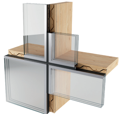
Schematic construction of a TGC façade
