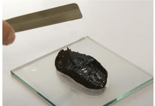
“chewing gum” consistency, the sealant shows resetting behaviour → mixture has already reached its pot life
