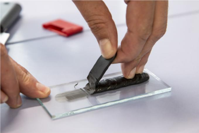
→ Peel off the adhesion strip and evaluate the appearance of fracture!
