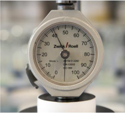
→ Determination of shore-A hardness by a durometer!
