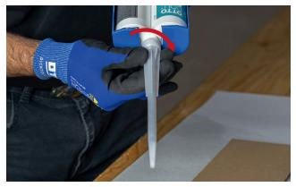
Clean off material and screw on static mixing nozzle
