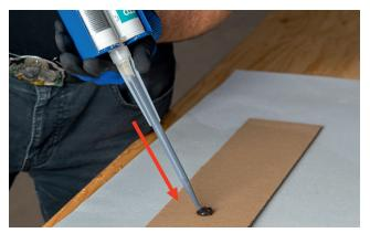
Refill the static mixing nozzle with adhesive and check the homogeneity of the mixture (see the quality checks for 2-component products to be carried out during processing)
