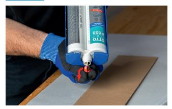
Insert the cartridge into the gun tray, unscrew protective cap and remove plug
