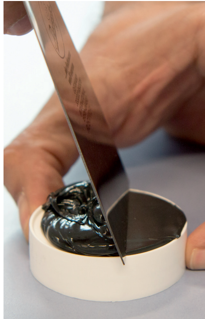
Pull sealant off smoothly
