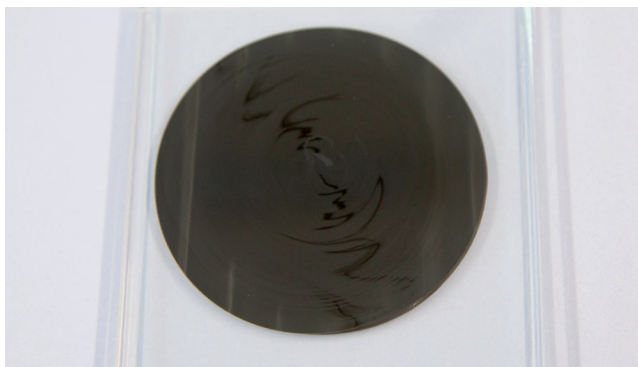
Glass plate test – Expected mixing pattern during cartridge processing
