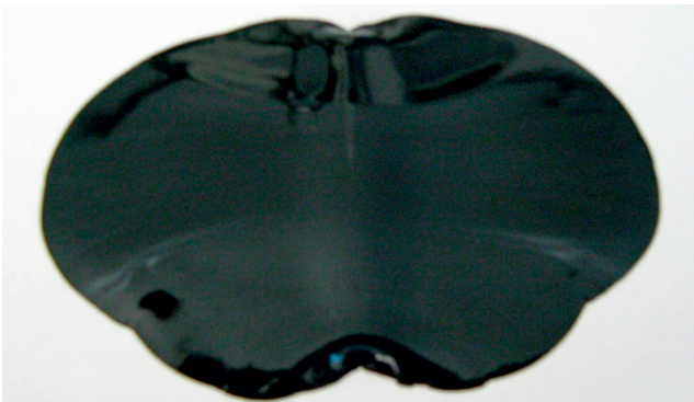
Pull paper apart - Expected mixing pattern during cartridge processing
