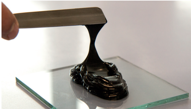
Paste-like consistency, spreadable -> Pot life has not yet been reached
