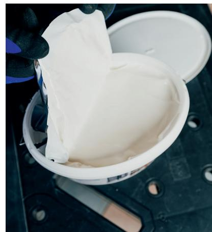
After opening the container, remove the packet of silica beads and then, starting at the container edge, pull off the film and remove any hardened material if necessary (do not stir in!). If the adhesive is not needed in its entirety, save the silica bead packet and the film for resealing later.
