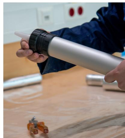
When processing OTTOCOLL® M 595 in aluminium foil bags, a hand-operated or accumulator gun suitable for foil bags can be used. To do this, open the aluminium foil bag, place the bag nozzle on top and insert the aluminium foil bag with bag nozzle into the gun. Alternatively, the desired amount of adhesive can be spread directly from the aluminium foil bag onto a spatula. Further processing is then carried out using a toothed spatula.
