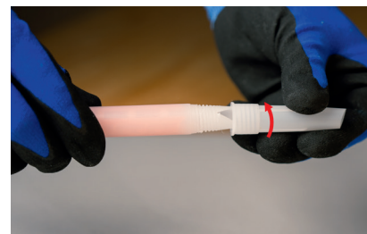
Screw the standard nozzle for cartridges onto the static mixing nozzle for BlueLine cartridges as far as it will go
