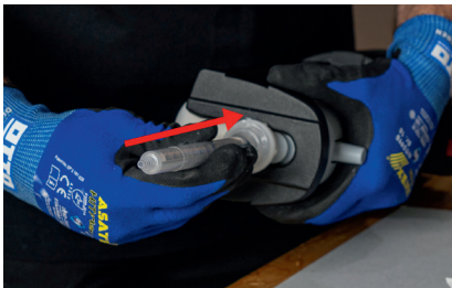
Wipe off the material and fit the OTTO static mixing nozzle ACF ORBIS 12-24X 10:1
