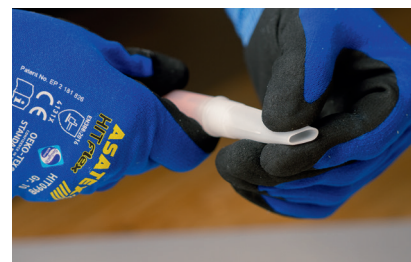
Standard nozzle flattened
