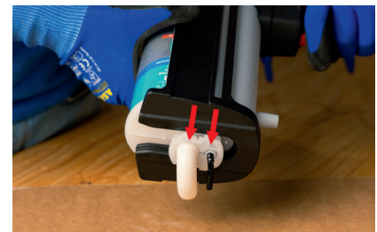
Press out the material without the static mixing nozzle until it escapes from both openings
