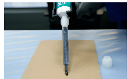
Check the bead discharge and the homogeneity of the mixture (see the quality checks for 2-component products to be carried out during processing)
