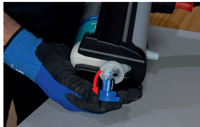
Unscrew and remove the plug
