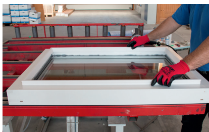
Insert the glazing bars
