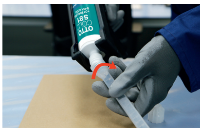
Wipe off the material and screw on the OTTO static mixing nozzle MGQ 10-16D as far as they will go
