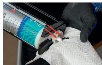
Press out the material without the static mixing nozzle until it escapes from both openings
