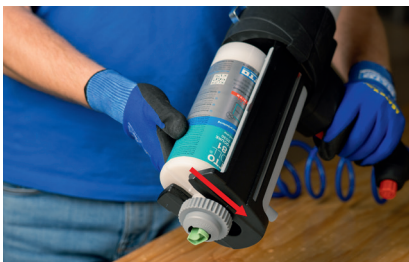
Insert the BlueLine cartridge into the gun
