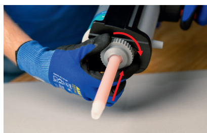
Fix the static mixing nozzle with the union nut
