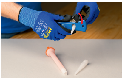
Shorten the standard nozzle as required before screwing it on
