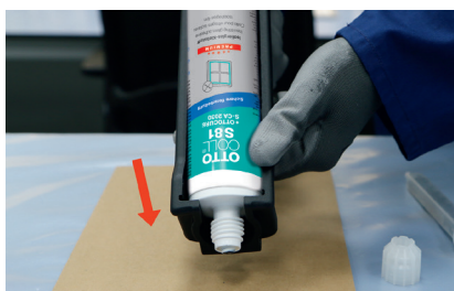
Insert the coaxial cartridge into the gun
