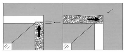
The jointing tape must not be applied around corners and when calculating the length of tape to be fitted add 1 cm/m to the actual joint length. The tape is equipped with a thin adhesive coating, through which overstretching will be avoided. Assemble the tape without stretching. For connections of the tape in long joints, make a close butt connection (oversize in length).
