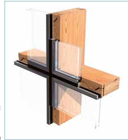
Design of timber-glass composite units
