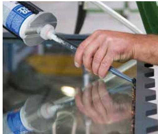
Applying the 2C silicone for wood-glass composite elements
